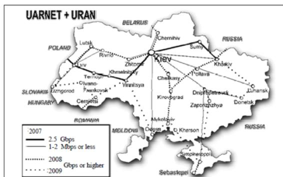
Fig. 1. Fiber optic channels for UNGI
